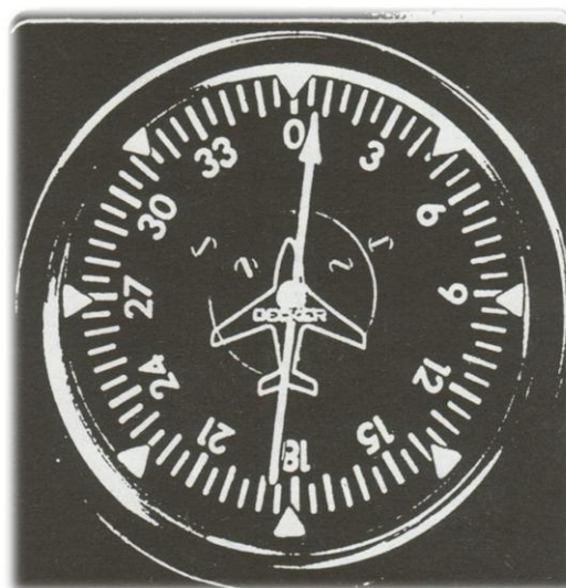
Abb. 13 RBI; Relative Bearing Indicator
